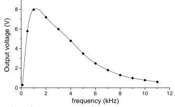
Fig. 2. The relative frequency response of the VLF receiver.
